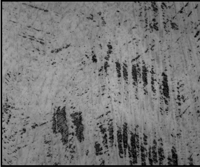
Fig. 10 — Microstructure of weld 65N1716-4R after bending. Diluted Kane's Etch, X200. Magnetic response equal to that of 0 FN before bending and 4.5 FN after bending indicates a small amount of martensite formation during bending. The dark etching regions contain some martensite. No ferrite is present.
